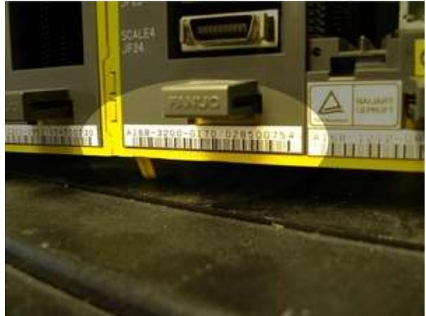
The mainboard Part Number is located at the bottom of the second last board on the control. See close up above.
